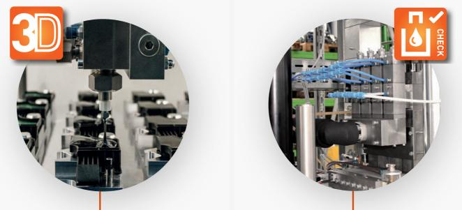
Most dosing supervision systems only detect a fault in the filling quantity during casting, thus generating unnecessary waste by casting errors. The new **HEDRICH PreCHECK**<sup>™</sup> system, however, recognizes improper dosing of the cast resin components yet before casting. Therefore, waste is avoided.
